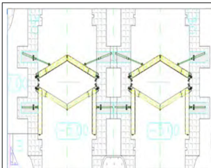
Figure 3-5. Ship lock gate with two layers of the “X-shaped”- stage of feasibility study
