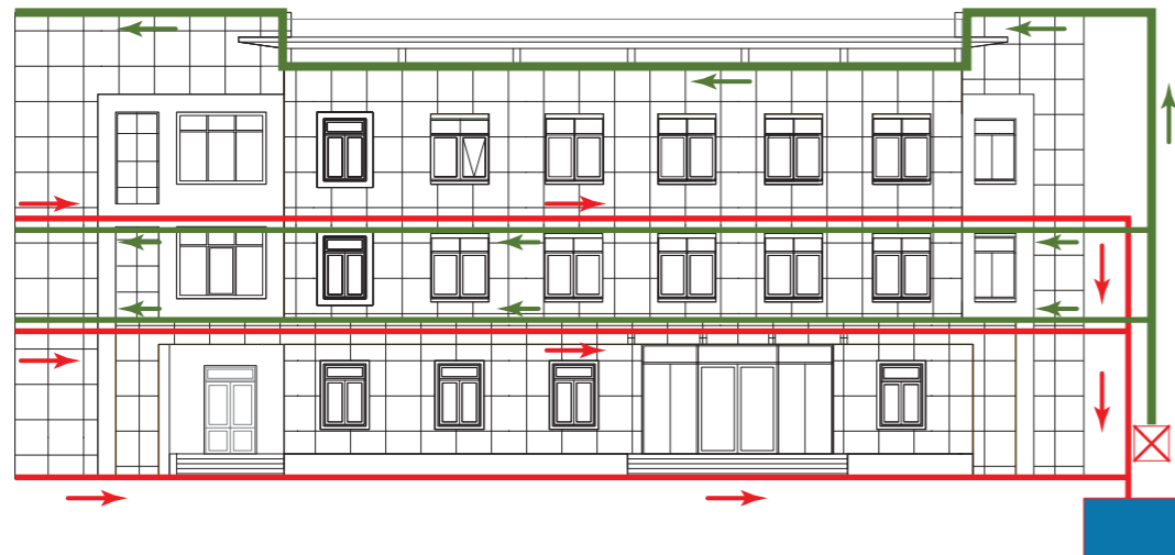
Figure 33: The irrigation system design of the green walls Source: © GIZ/VN-SIPA Project
